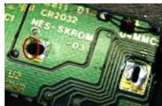
**Step 3:** Install a battery into the clip and dry fit it into the PCB. Make sure it sits as low to the PCB as possible. Try setting the PCB back into the case and see how it fits. Depending of the PCB / location of the battery, the clip may bump into a standoff inside the case, in
