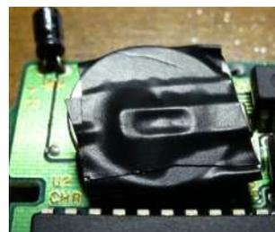
**Step 3:** Wrap each end of the tape up over the top clip, pulling somewhat snugly to ensure a tight connection.
