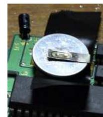
**Step 2:** Insert the new battery in between clips, with the positive (+) side up.
